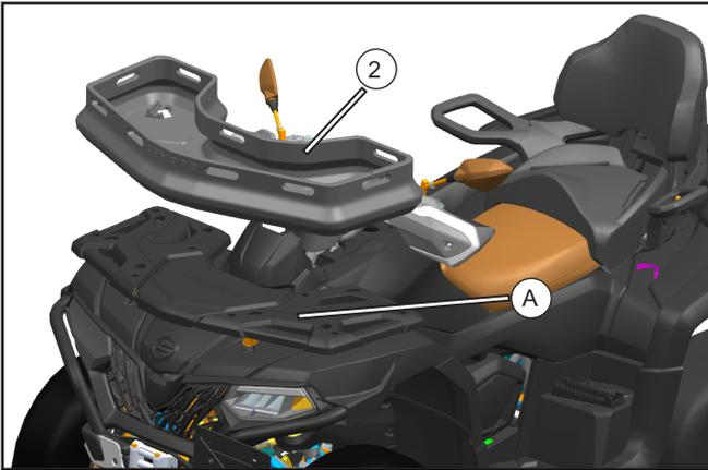
// Place the cargo basket (2) on the front rack cover (A) of the vehicle , and align 4 CF Connect clamp holes.
