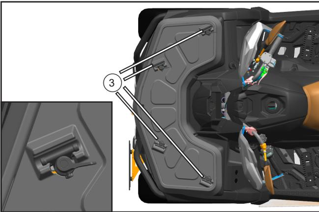
// Install the CF Connect clamps (3) and tighten them by turning the lever clockwise.
